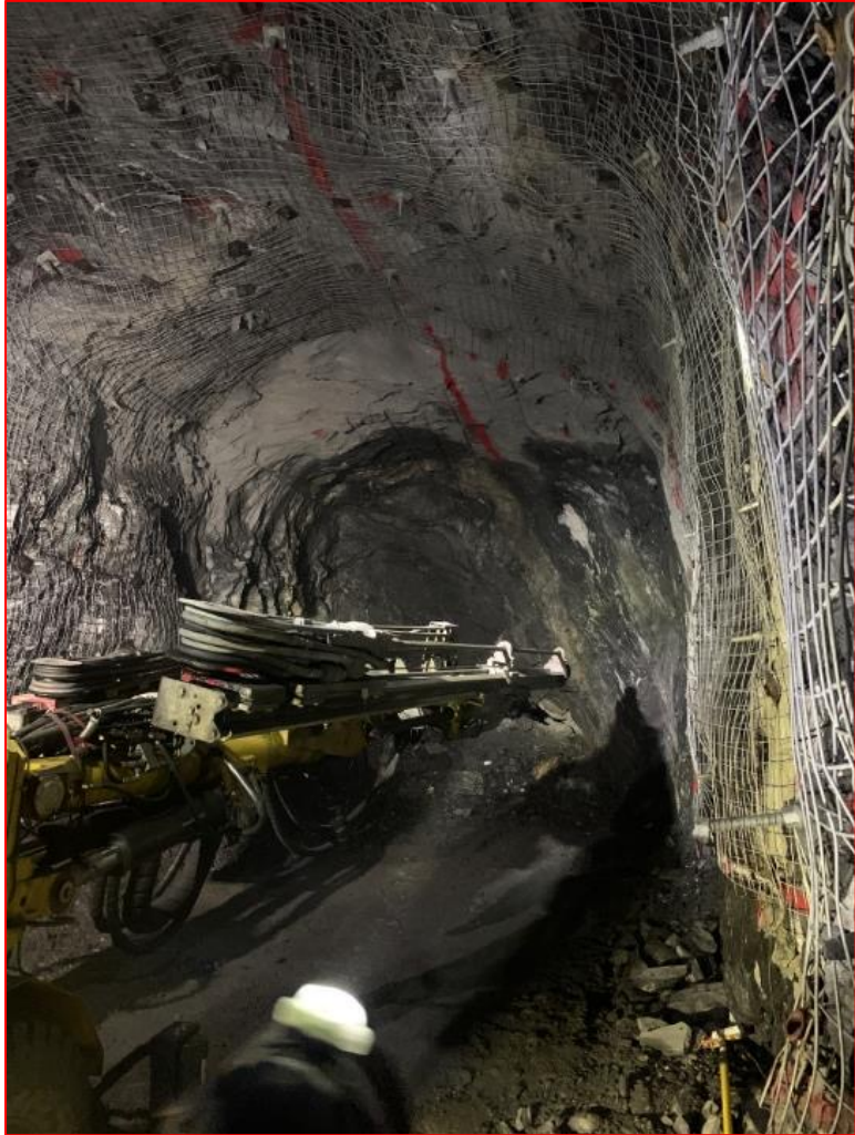
Scaling the Drift with the Jumbo
