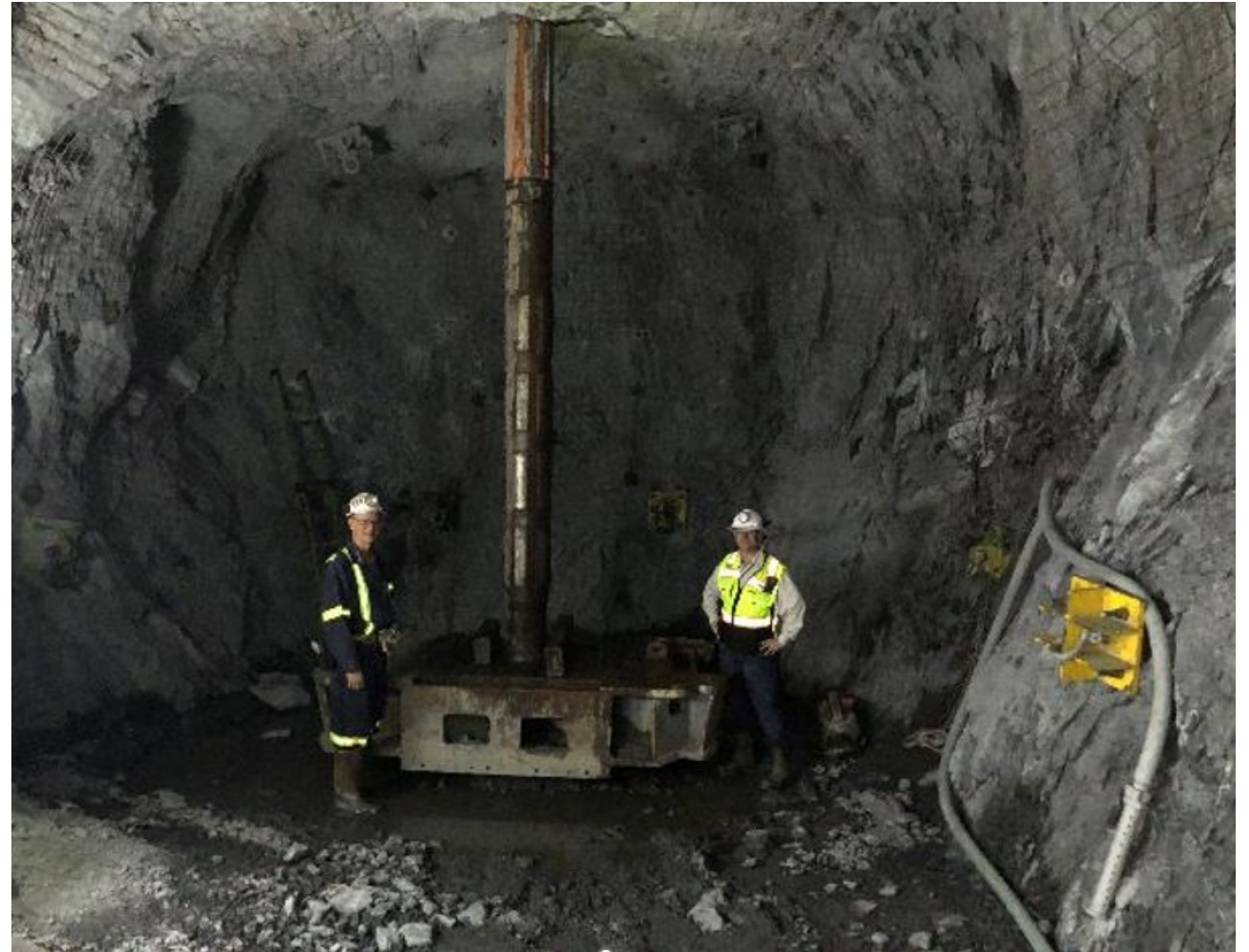
Raise Bore Cutter Head / Reamer (Break Through)
