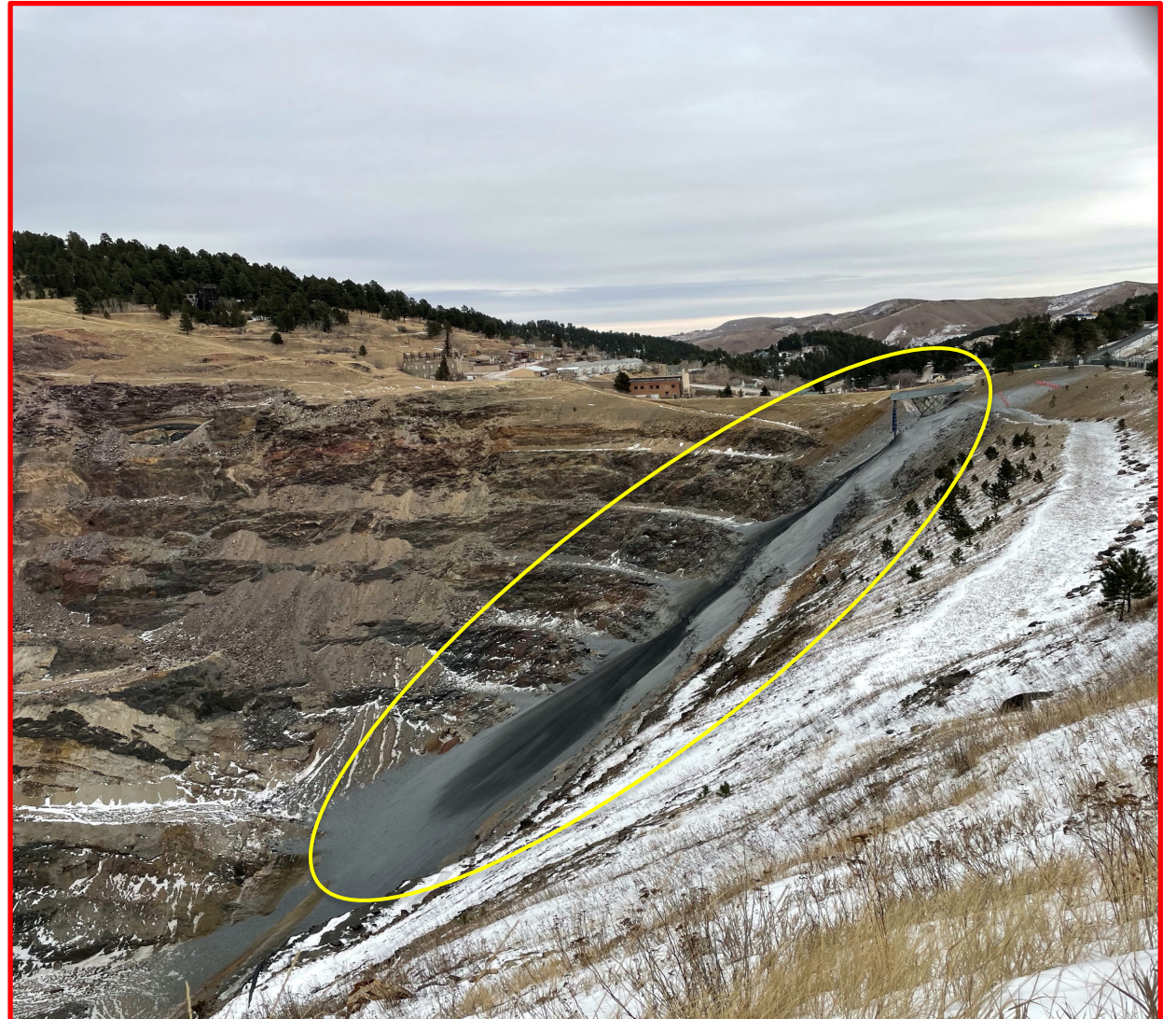
Stockpile treated with tackifier is shown as the dark color; untreated stockpile is shown as the light grey color which is causing the dust issues.
