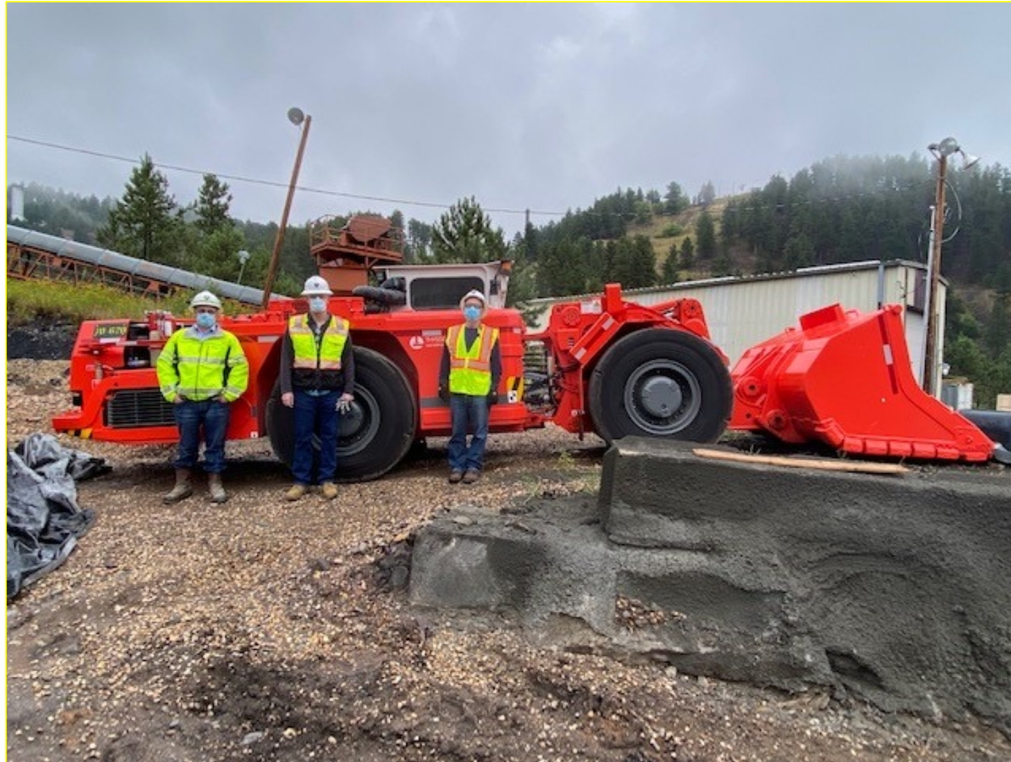
4 CY Mucker to be disassembled and mobilized to 4850L
